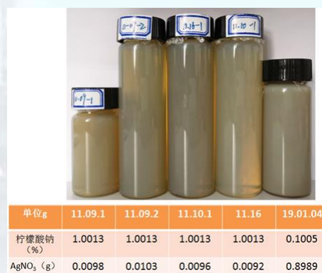
Fig. 5. Sodium borohydride reduction of silver nitrate.
