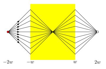
A parallel slab of ideal backward material. It maps the upward object at the left into an equally large upward image at the right. No diffraction limitation!
