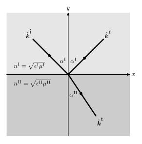
Incident, transmitted and reflected beam at interface of normal materials
