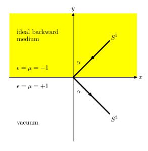
Power flow of a a beam which passes from an ideal backward medium to vacuum.
