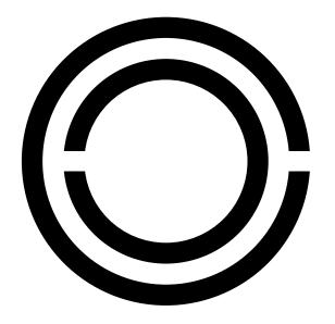
The split ring resonator. Inductance L and capacitance C. Resonance frequency is  $\Omega = 1/\sqrt{LC}$ .
